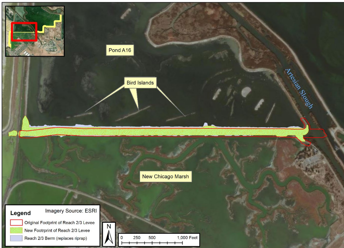
Figure 3. Reaches 2 & 3 Updated Levee Footprint and Sacrificial Berm
